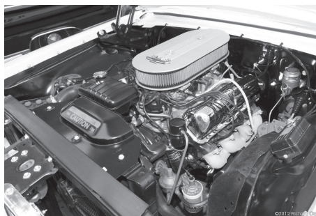
Dual Quad 427 cid Ford V8 power under the hood of the R-Code lightweight Galaxie
