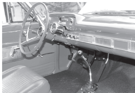
Four-speed T-10 manual gearbox with Hurst shifter and steering column mounted tach
